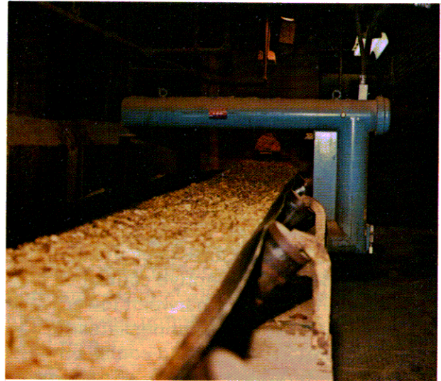
Continuous measurement of chip weight and moisture contribute to significant reductions in Kappa test variations.
